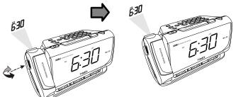
5. If you do not want to see the projected image, press the **PROJECTOR ON/OFF button** to switch the projector 'Off'.
